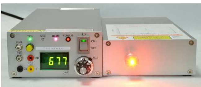
with Orange Laser 20mW output at 677mA, maximum upto 700mA.
