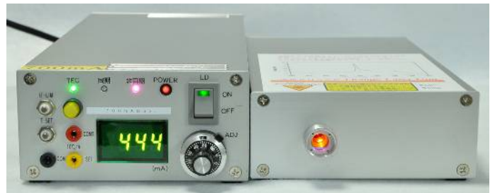
with Orange Laser 20mW output at 677mA, maximum upto 700mA.
